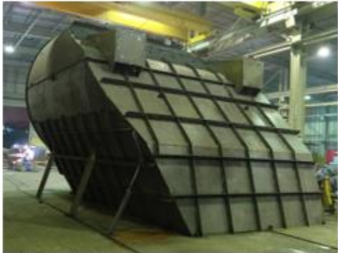
Fabrication of new duct Supplied to Al-Yammamah Cement Plant
