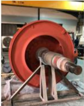
Repair of Cooler Fan Impeller For Qassim Cement Plant
